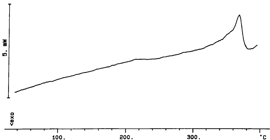
FIGURE 5 Thermal analysis of polyester 2b monitored with 20 K/min.
